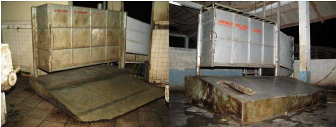
Figure 01 Mark I restraining boxes showing lower plinth height (left figure) and modified box with raised plinth (right figure)
