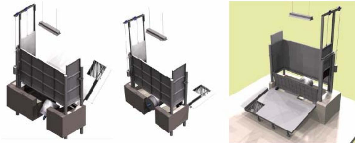
Figure 02 Mark II restraining box showing side wall in its final resting position (right figure)
